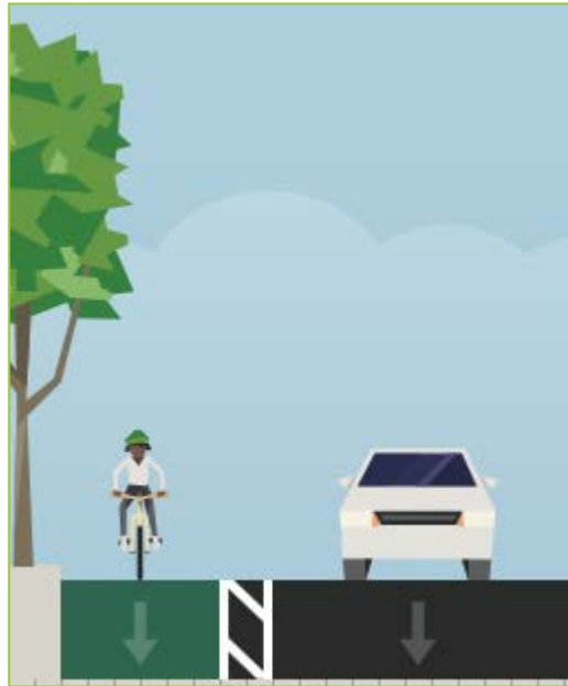
Marked/Buffered Bike Lane
