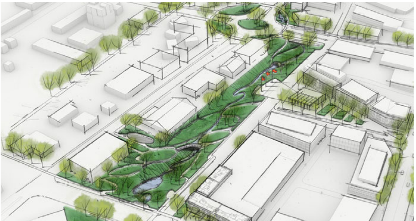
Water management area buffering the Mixed-use Village Core from the Maker area. While creating more green open space, this area can improve the resiliency of the North End area by absorbing and retaining excess water during intense rain events.
