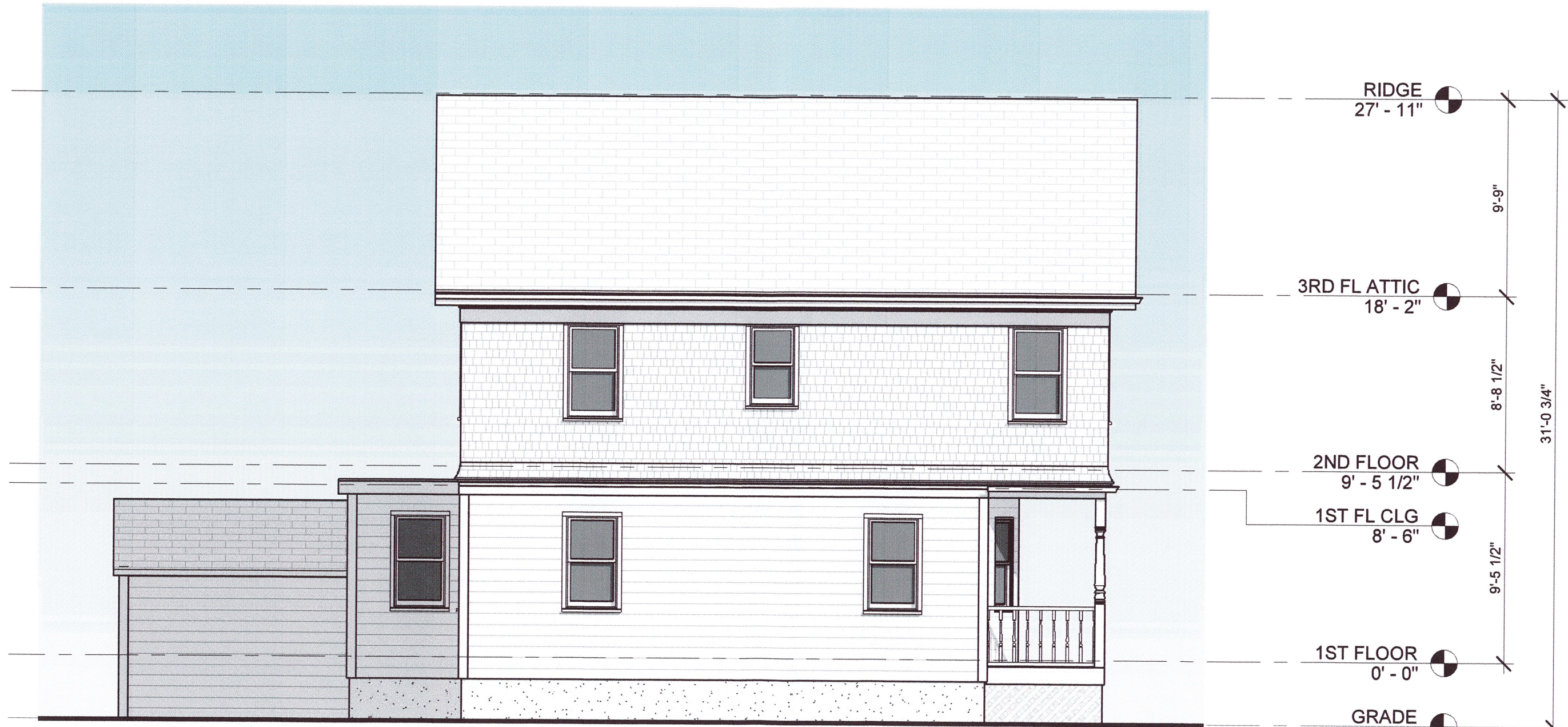
1 EAST ELEVATION EXTG 3/16" = 1'-0"
