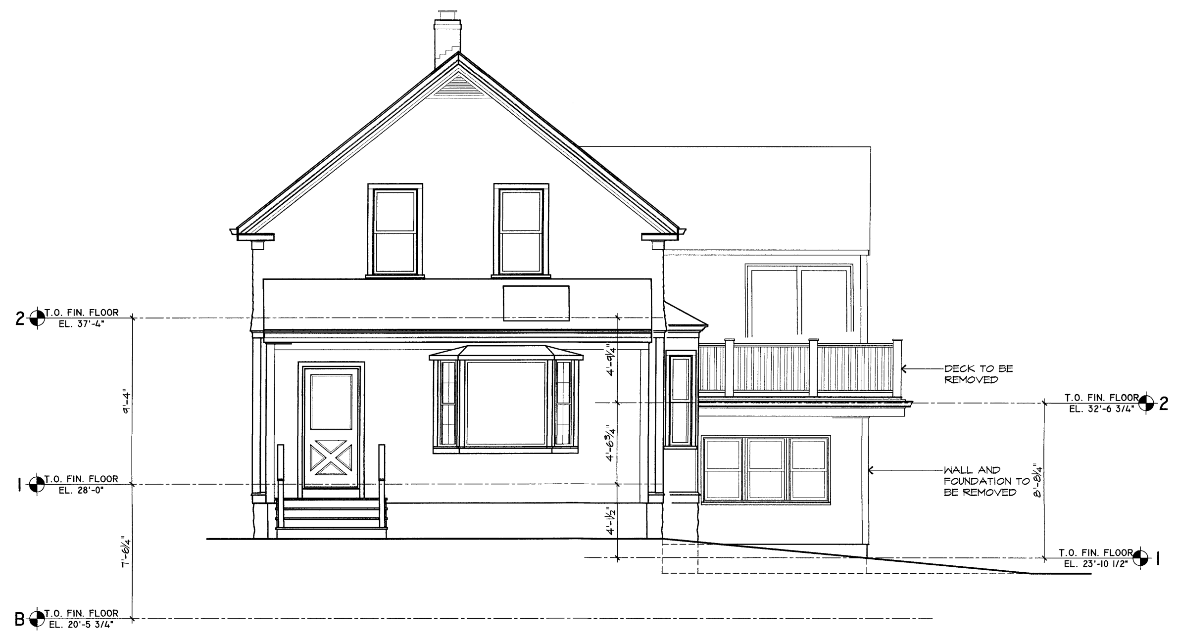
EXISTING WEST ELEVATION ROSENEATH AVENUE SCALE: 3/16" = 1'-0"
