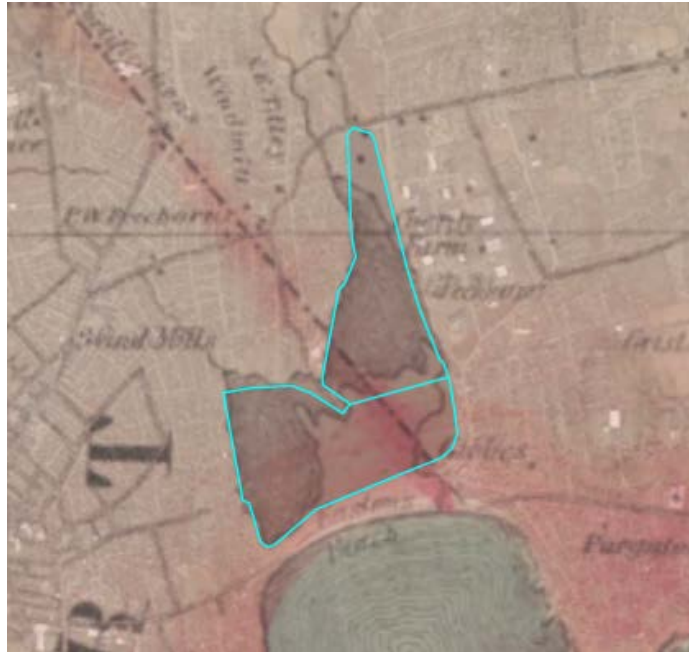
Figure 4: Footprint of the North and South Easton Pond Dams over former low-lying marsh areas.
