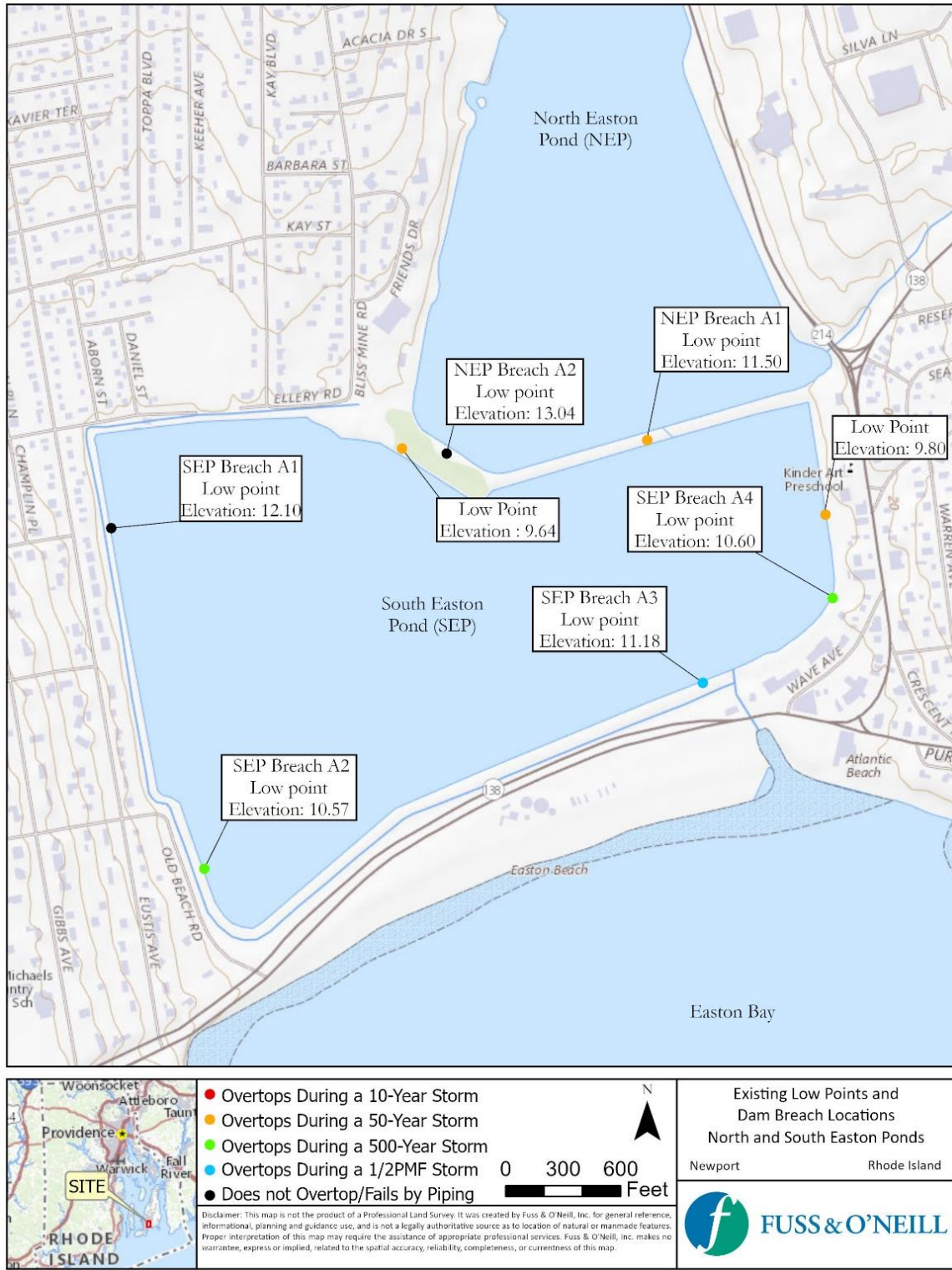
Figure 13: Modeled dam breach locations and existing embankment low points at NEP Dam and SEP Dam
